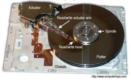
As can be seen in the above picture, the desktop hard drive has six components: the head actuator, read/write actuator arm, read/write head, spindle, and platter. On the back of a hard drive is a circuit board called the disk controller.
